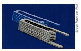
Researchers at Fraunhofer IFAM have developed a technological casting process that enables the production of lightweight windings made of aluminium with a high slot fill ratio. A study has now shown that aluminium coils increase the continuous output of electrical machines compared to copper windings, reduce the operating temperature and at the same time save weight and raw material costs.
